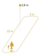
Possible mounting height: 2,00 m - 4,00 m Orange: radial and tangential
