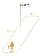
Possible mounting height: 2,00 m - 4,00 m Orange: radial and tangential
